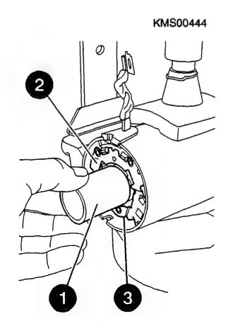
Assembling commutator end shield
